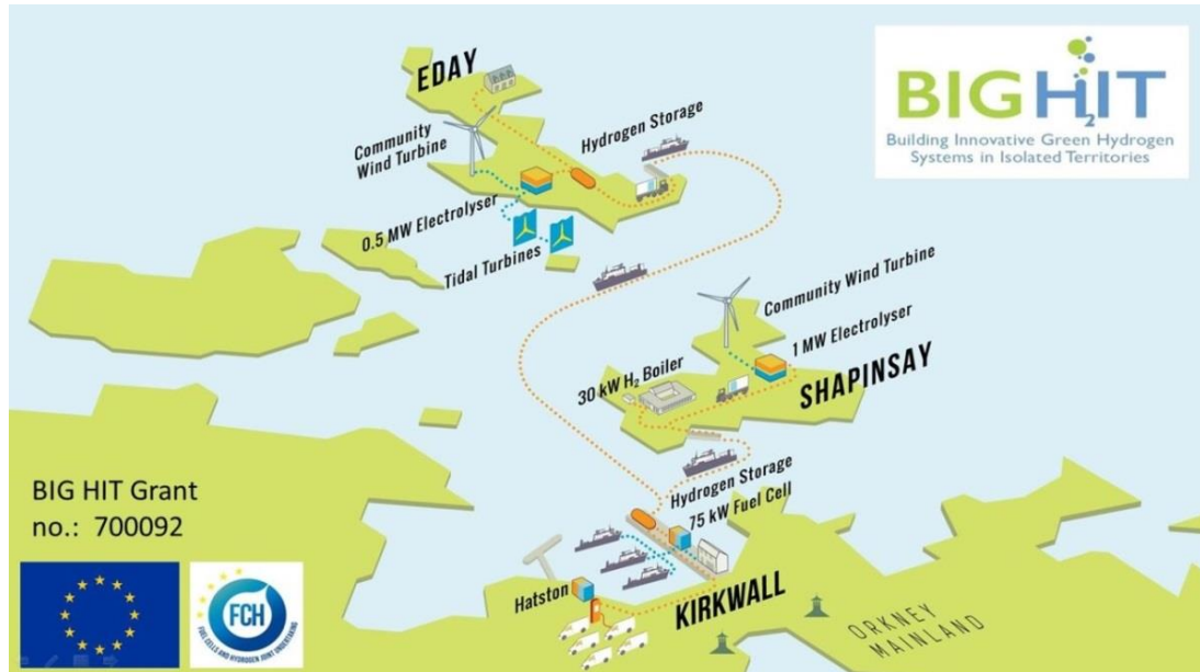
Figure 1. Schematic of BIT HIT project in the Orkney Islands
