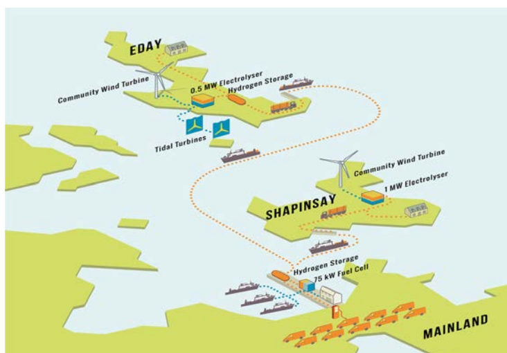
Figure 2 Schematic of BIG HIT project in the Orkney Islands
